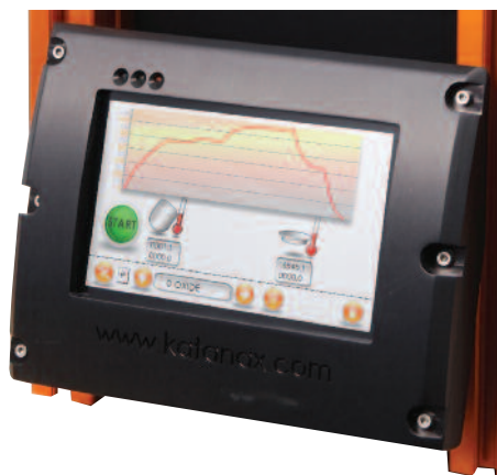
Illustration of a fusion program in graphical form. This allows you to see all of the fusion parameters in a easy to understand format.
