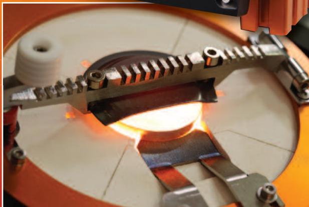
K1 furnace controls the temperature to +/- 1 degree during the fusion process
